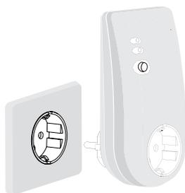
Insert the heater's shockproof plug into the wireless plug socket receiver X3D for the power supply.
